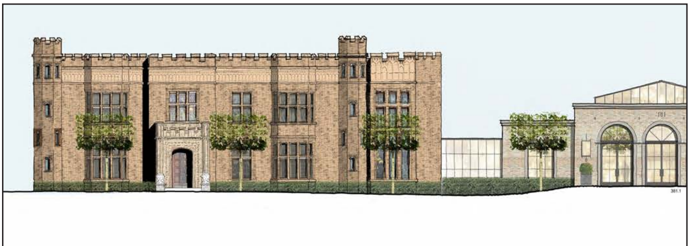
FIGURE 7. FRONT FACADE SHOWING EXISTING ABBEY AT LEFT AND NEW ENTRANCE AND 2-STORY WING AT RIGHT
